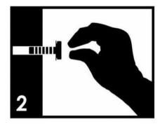
Position each part correctly and insert screws or bolts into their respective holes by hand tighten or using the proper hand tool. Only tighten when step is completed or when instructed to do so.
