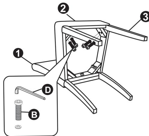
Put the screws in the holes, tight the screws,
